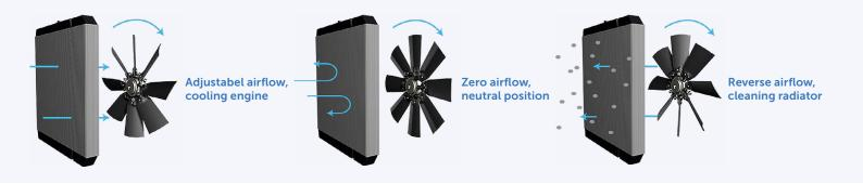
Reversing happens at full speed by hydraulic or pneumatic actuation of the internal cylinder, rotating the fan blades instantly from a working position, over the neutral, into reversing and back.
